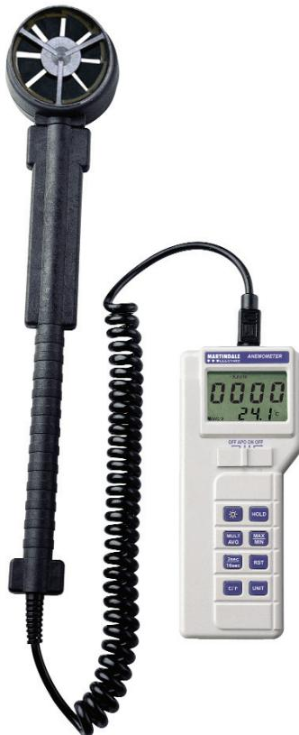
This meter displays temperature ( $^{\circ}\text{C}$  or  $^{\circ}\text{F}$ ) and airflow at the same time. Maximum and minimum figures for flow and temperature can be shown. For more accurate measurements, up to 8 readings can be taken and automatically averaged.
